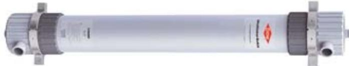
Systems designed with Ultra filtration use an outside-in flow configuration which allows for less plugging, higher solids loading, higher flow area and easy cleaning. The primary flow design is dead-end filtration but the module can be operated using a concentrate bleed. Dead-end filtration uses less energy and has a lower operating pressure than the concentrate bleed, therefore reducing operating costs.
